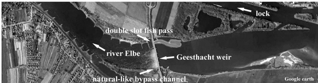
Figure 1. Position of the natural-like bypass channel on the left bank (undercut bank) and the double vertical slot pass on the right bank (slip-off bank) (source: Google earth 2012)
